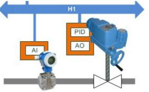
Figure 4: Example for process control
