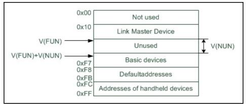
Figure 12: Device address range
