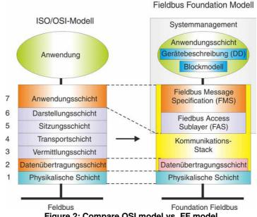
Figure 2: Compare OSI model vs. FF model
