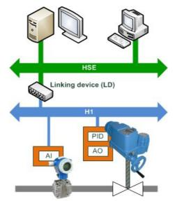
Figure 1: typical Foundation Fieldbus structure
