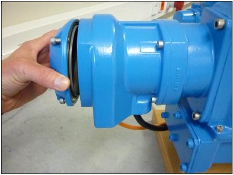
Figure 6: Terminal compartment for Foundation Fieldbus
