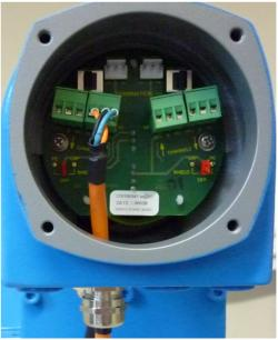
Figure 7: Bus connection board
