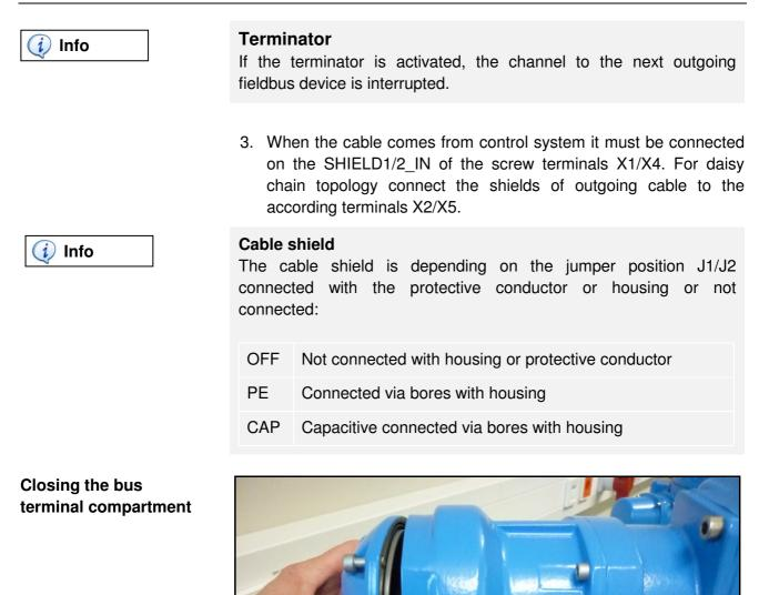
Figure 9: Terminal compartment for Foundation Fieldbus
