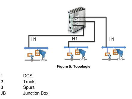
Spurs or tee connectors are possible for Foundation Fieldbus. The possible fieldbus line length is determined by the type of cable, the cross section, and the type of the bus supply.
