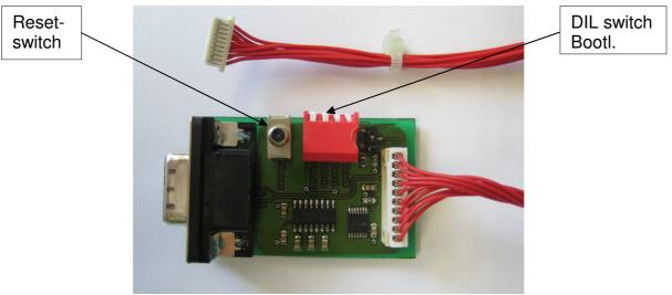
Signal level converter RS 232-TTL
