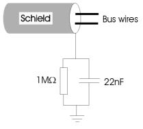
High impedance grounding of shield
