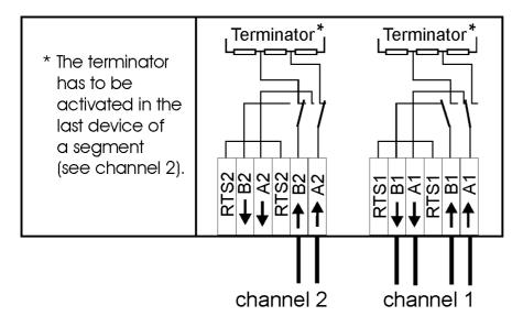
example for termination with slide switch S3, S4 on DiM-19 connection board
