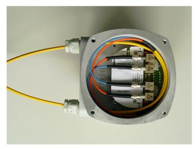
Fibre optic connection inside the compact plug
