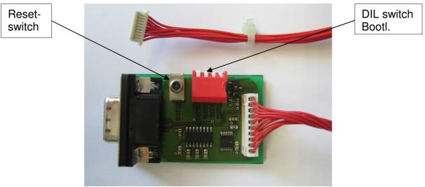
Signal level converter RS 232-TTL
