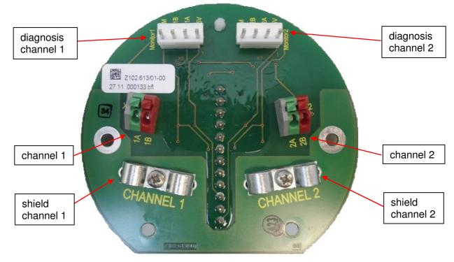
Connection board for modbus loop topology:
