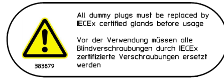
Label with warning for actuators of explosion-proof version IECEx type
