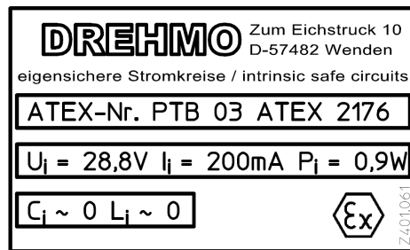
Label for intrinsic safe circuits with EM7.005
